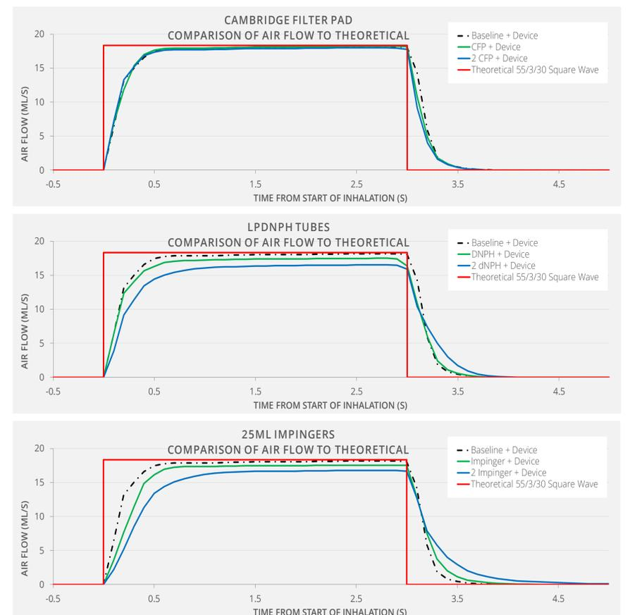
Figure 3: Typical Airflow profile with Hypothesised Causes for Distortion
